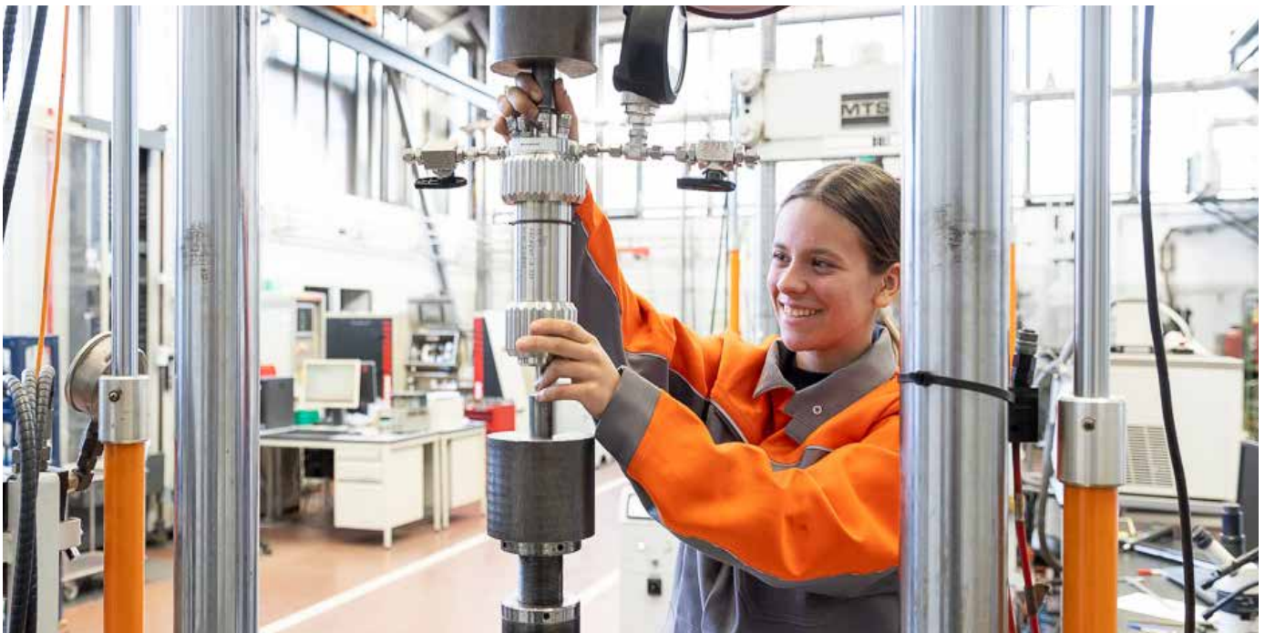
Tensile test rig with H 2 -Autoclave
