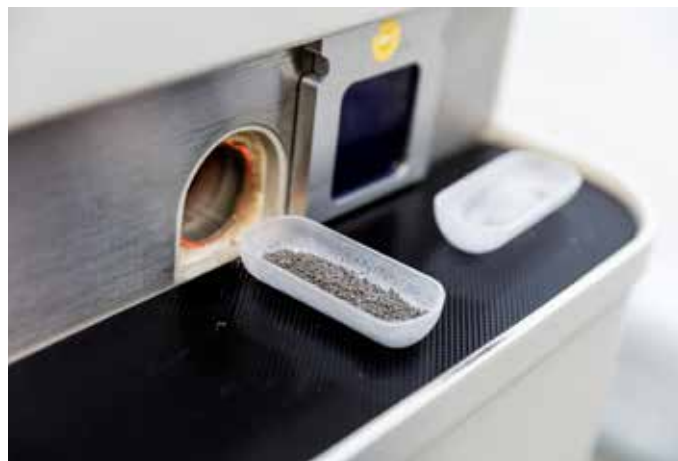
Sample before carrier gas hot extraction and red-hot sample during the measurement
