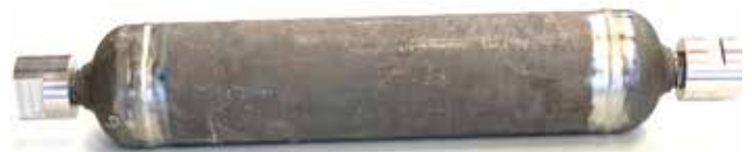
Example of a vessel prepared for burst test
