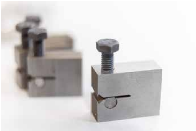
K_{IH} test specimens with bolts to apply constant displacement
