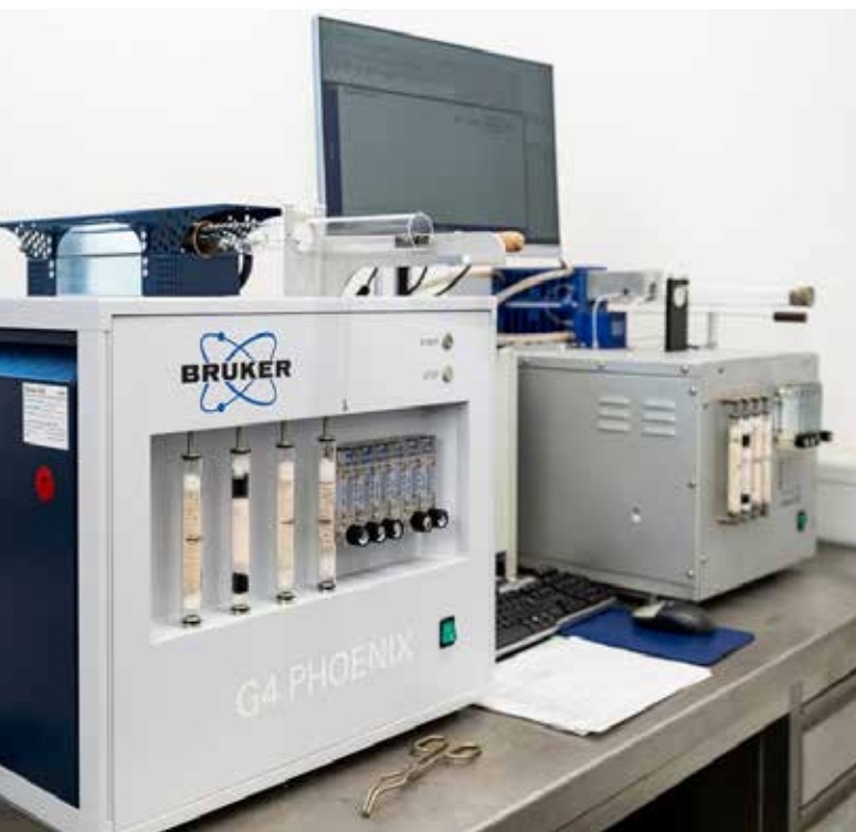
For carrier gas hot extraction we apply Bruker G4 Phoenix
