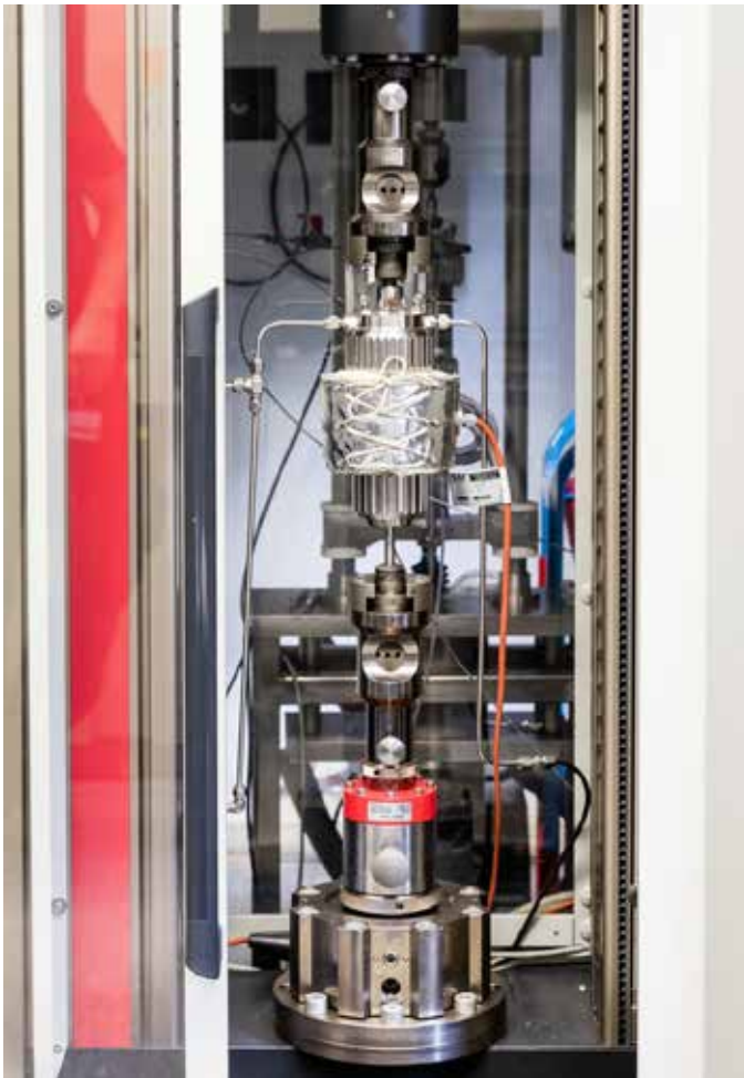
Tensile test rig for SSRT with H 2 -autoclave
